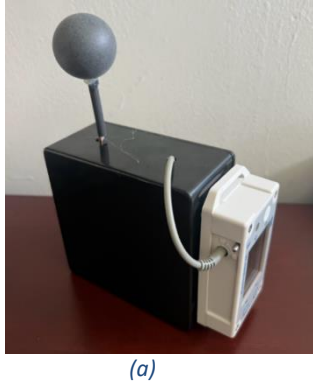
Figure 1. The two sets of instruments that were used: (a) the WBGT logger and (b) the Wi-Fi logger
